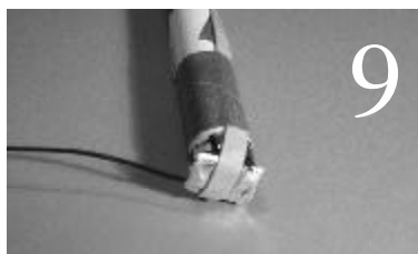
9. Tuck the foil under the rubber band. Repeat for the other end of the battery.
