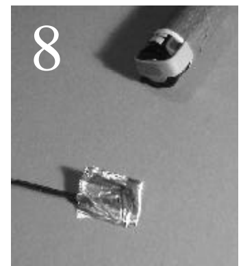
8. Fold the package in half so that the wire inside is also bent in half, to keep it secure.
